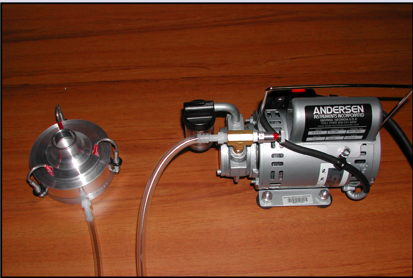
Anderson Single Stage Impactor with pump (1-STG) for collecting air samples. The sampler is rated to capture airborne particles down to 2µm in diameter.
